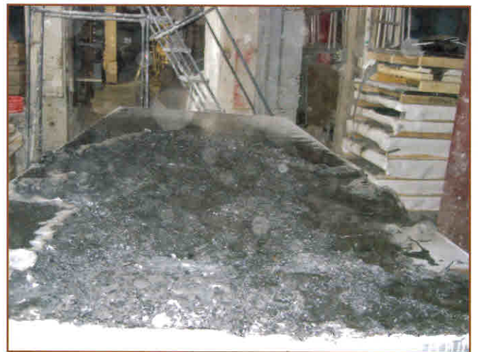
Photo 7 – FR-rated EPDM over isocyanurate, showing excessive lateral flame spread on both sides.
