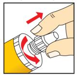
1. Remove twist cap from the top of the cartridge.
