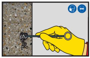
Repeat the cleaning procedure before proceeding to the next step. In other words, repeat steps 2 and 3 and then step 2 again before moving on to step 4.
