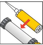
4. Place the cartridge into caulk gun when ready to start installation.
