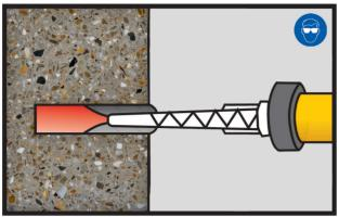
6. Insert clean, contaminant-free, dry, steel threaded rod or steel reinforcing bar for anchor installation.
