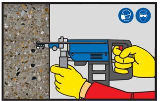
Ideally, the inside surfaces of an anchor hole need to be as clean, sound, dust-free and dry as possible prior to injection of an anchoring adhesive. A clean, damp surface can be tolerated, but an anchor hole should not contain standing water or have droplets of moisture clinging to the surfaces. For performance reduction factors and design guidelines when anchoring into water saturated or water filled anchor holes, please consult the current IAPMO UES Evaluation Report 601 (ER-601).
