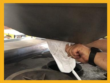
We put safety first by designing the SikaColor<sup>®</sup>-120 G 404 Series so that the supersacks can be untied while the cradle sits firmly on top of the machine.
