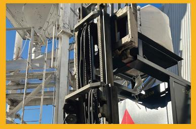
Loading totes of color is easy with the SikaColor<sup>®</sup>-120 G 404 Granular Color Dispensers. Simply place the tote onto the supplied cradle (left above), and then place the cradle atop the machine, where it slides in between metal guide rails (right above).
