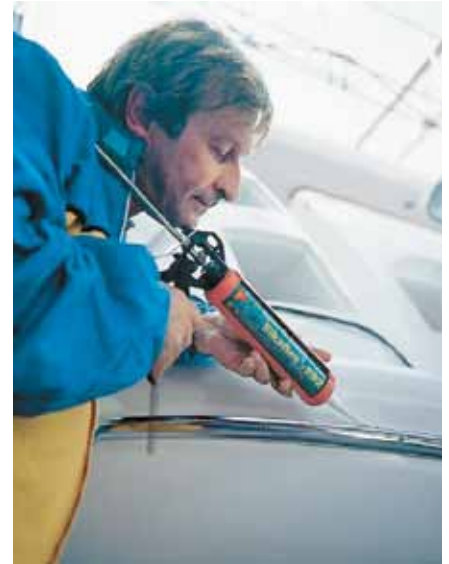
Fig. 78 Sealing the edge of a chrome rub-rail
