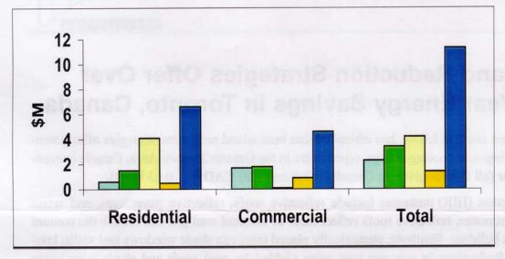
Savings in annual heating and cooling energy-use expenditure assuming a uniform residential and commercial electricity rate of \$0.084/kWh and a gas rate of \$5.54/GJ.
