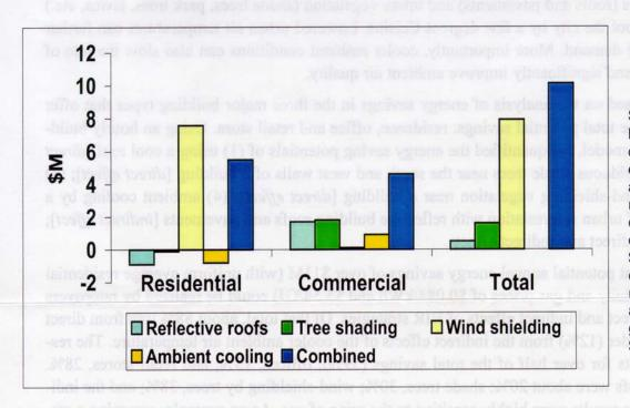
Savings in annual heating and cooling energy-use expenditure assuming a uniform residential and commercial electricity rate of \$0.084/kWh, a commercial gas rate of \$5.54/GJ, and a residential gas rate of \$10.84/GJ.
