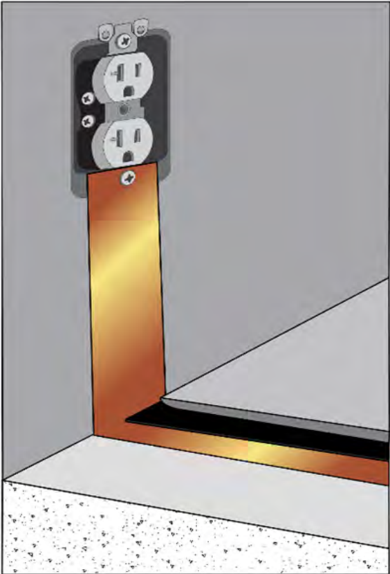
Ground to an ESD Electrical Outlet
