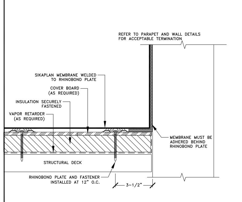
NOTE: DO NOT INSTALL RHINOBOND PLATES TIGHT AGAINST WALL. THE RHINOBOND WELDER IS 7" WIDE AND MUST BE CENTERED OVER THE RHINOBOND PLATE FOR PROPER WELDING.
