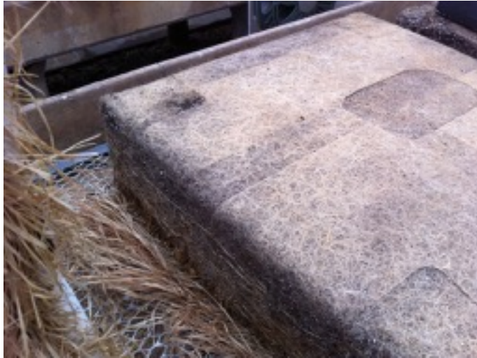
FIGURE 5. TYPICAL ROOT MAT OBSERVED ON THE BOTTOM OF THE SARNAFIL MEMBRANE TEST BOXES
