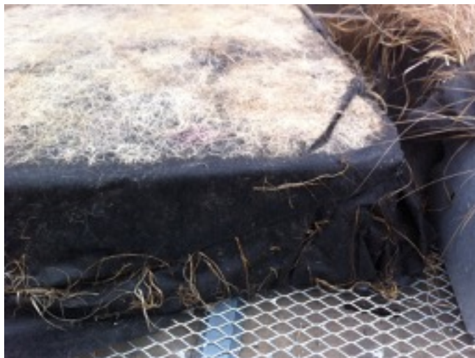
FIGURE 2. TYPICAL CONTROL ROOT MAT AFTER THE TEST BOX WAS REMOVED WITH THE FABRIC LAYER STILL ATTACHED
