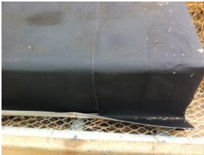
FIGURE 4. OUTER MEMBRANE SURFACE OF TYPICAL SARNAFIL G 410 MEMBRANE AT HARVEST.
