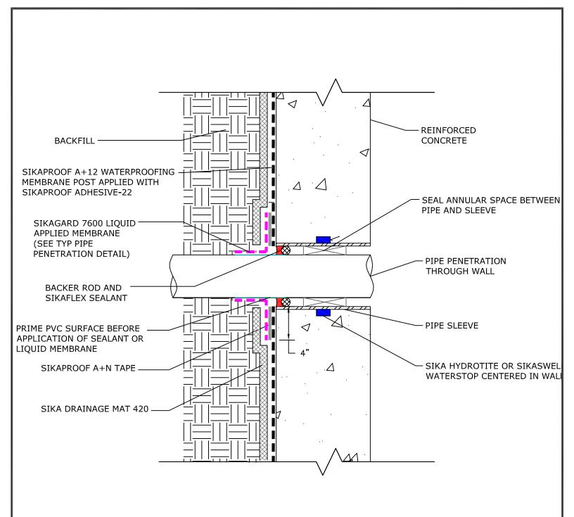
NOTE: DETAIL CAN BE USED FOR HORIZONTAL OR VERTICAL APPLICATIONS
