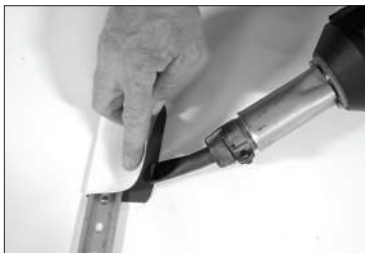
Welding protection pad
