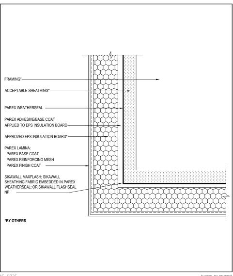
Ensure Parex 355 Standard Mesh, SikaWall Intermediate 6 or SikaWall Intermediate 12 Reinforcing Mesh is lapped a minimum of 8" (203 mm) around corners.
