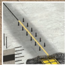
Leaking movement joints
