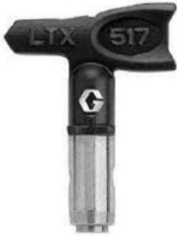
Many tips are reversible for self-cleaning. If clogged, engage trigger lock, reverse tip, disengage trigger lock and pull trigger to pump coating through orifice at high pressure to blow out dried/clogged material.
