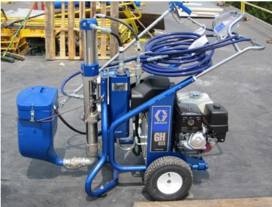
A typical airless pump sprayer. A gas powered, hydraulic sprayer shown here is capable of dispensing up to 4 gallons per minute.
