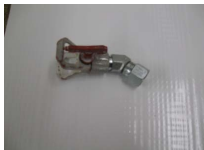
An extension wand can be added to most guns to make spraying more comfortable and to keep the spray away from the operator. A swivel tip allows for proper angling of the spray pattern.
