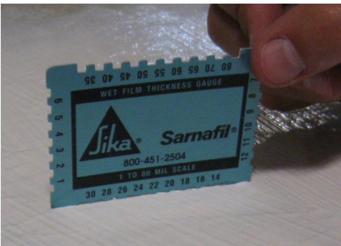
To achieve 133 – 100 ft<sup>2</sup>/gal (3.3 – 2.5 m<sup>2</sup>/L) coverage the wet mil thickness of the adhesive should be approximately 12-16 mils wet.
