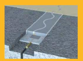
Sika FloorJoint panels are well-suited to new building construction as well as restoration of defective joints in existing facilities. Sika's rapid curing resin systems bond the panels securely to the concrete substrate, which speeds installation to minimize downtime and the interruption of operations.
