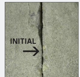
SikaControl®-245 WT Liquid Sealed Hairline Crack
