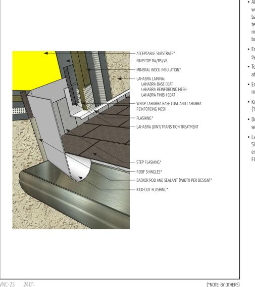
• All terminations must be fully encapsulated with mesh reinforced base coat. Prebackwrapping is recommended at drainage terminations. Extend reinforcing mesh a minimum of 2 1/2" onto back of insulation board.
