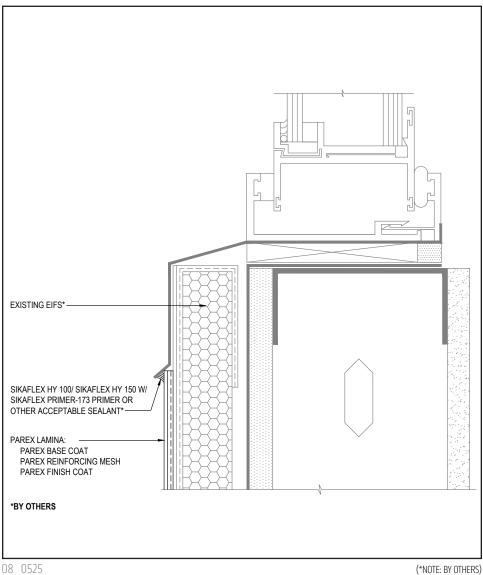
• Seal flashing with Sikaflex HY 100 Sikaflex HY 150 with Sikaflex Primer 173 or other acceptabl sealants. Reference Acceptable Sealants for use with Parex Wall Systems Technical Bulletin for a list of sealants.
