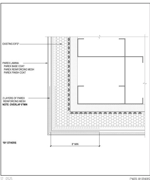
• Ensure Parex 355 Standard, SikaWall Intermediate 6 or SikaWall Intermediate 12 Reinforcing Mesh is lapped a minimum of 8" (203 mm) around corners from both sides (creating double layer of mesh at corner).
