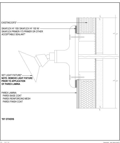
Use Sikaflex HY 100 Sikaflex HY 150 with Sikaflex Primer 173 or other acceptable sealants. Reference Acceptable Sealants for use with Parex Wall Systems Technical Bulletin for a list of sealants.
