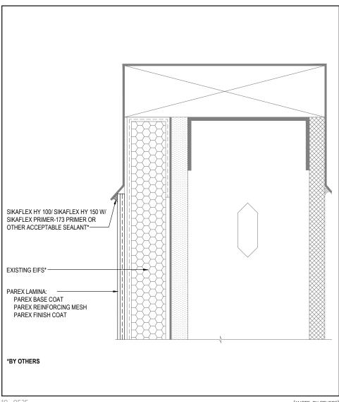
Seal flashing with Sikaflex HY 100 Sikaflex HY 150 with Sikaflex Primer 173 or other acceptable sealants. Reference Acceptable Sealants for use with Parex Wall Systems Technical Bulletin for a list of sealants.
