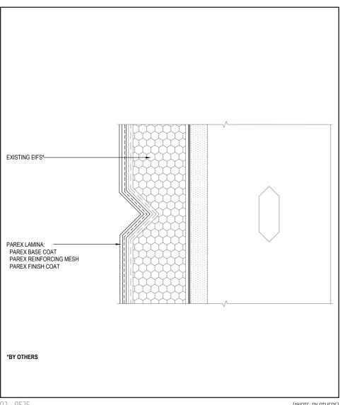
• Reinforcing mesh shall be continuous and care shall be taken to ensure reinforcing mesh is not cut during base coat application.
