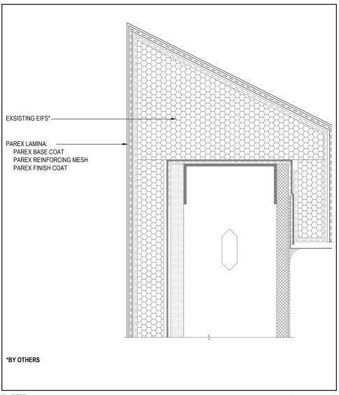
Do not apply Parex Lamina to flat horizontal surfaces. Provide a minimum 6:12 slope for all horizontal surfaces over 1".
