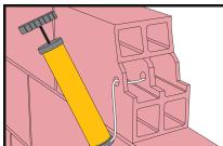
The drill hole must be cleaned after each cleaning step with a blow pump or by compressed air, starting from the bottom of the hole (pump at least 1x).
