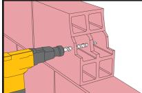
Drilling of hole with an electric drill to the diameter and depth required. Drill hole diameter must be in accordance with anchor and perforated sleeve size.
