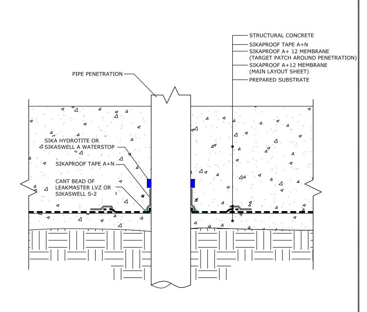
NOTE: DETAIL CAN BE USED FOR HORIZONTAL OR VERTICAL APPLICATIONS
