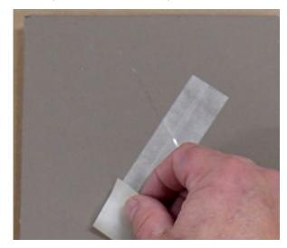
4. The tape is removed by grabbing the free end and pulling it off rapidly back on itself at a 180° angle, or as close to 180° as possible.
