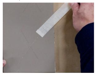
5. Compare the resulting amount of coating that is left intact to the levels included in ASTM D3359 for a rating. Note: Elcometer 99 Tape or other tapes qualified for use for ASTM D3359 testing may be used.
