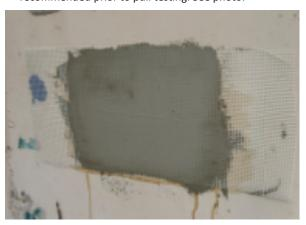
Once the test material has cured/dried, take the loose end of mesh or fabric and pull it straight out from the wall surface.
