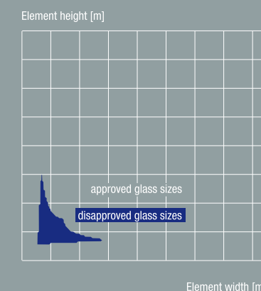
Fig. 6 Protective glazing, increase of seal height Glass: 10/12/8 + 8 mm, p_0 : 20 kPa Seal height: 18 mm
