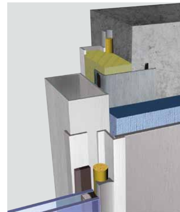
For wide gaps between the curtain wall and concrete structure SikaMembran® is the best solution.
