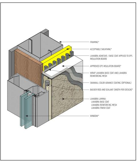
• All terminations must be fully encapsulated with mesh reinforced base coat.
