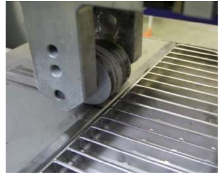
Edge-floor connection testing via WSTEC testing rig
