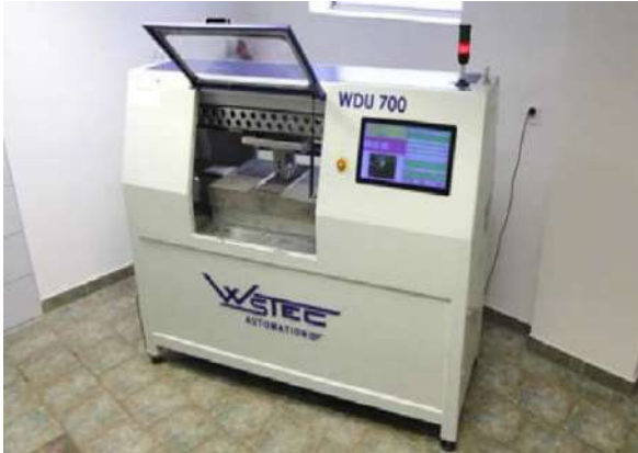
WSTEC rig developed for mechanical exposure testing
