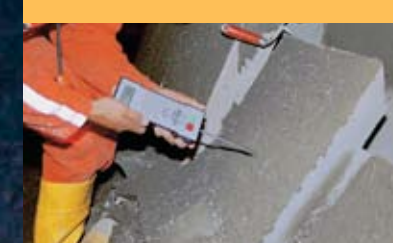
Early strength of 0 – 1 N/mm 2 Penetrometer method 3
