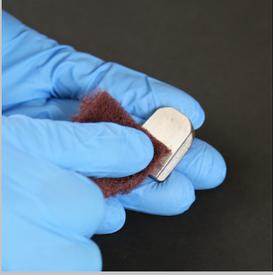
**1** Make sure all surfaces are clean, dry and free of dust or grease before bonding. For bonding plastic, metal, or paint, abrade bonding surface with Scotch-Brite™ pad or sandpaper (80 - 120 grit) and dry wipe to clean any debris.
