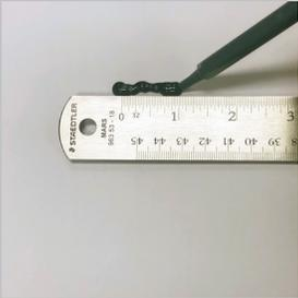
**4** Attach a static mixer. Purge 1" of material to ensure proper mixing.
