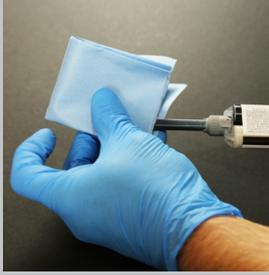
**6** After applying, a small amount of excess material may discharge from the static mixer due to back pressure. If this occurs, wipe excess material off mixer tip with paper towel. DO NOT pull back on the plunger as this may pull mixed material back into the syringe.
