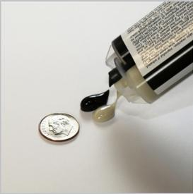
**3** Purge dime-sized amount of material to level plungers before attaching static mixer.
