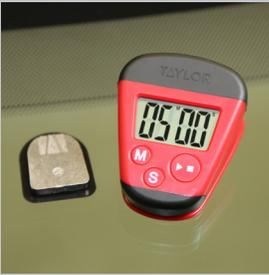
**8** Allow 5-10 minutes for material to set, afterwards the bonded part will be ready for use<sup>1</sup>. Product fully cures in 24 hours at 73°F.
